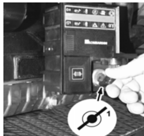
1st position - Warning light on.
